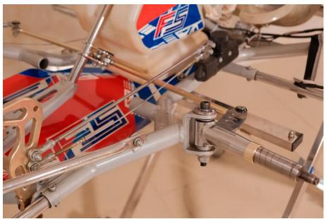
(2) Straighten the steering wheel and lock in the center if possible.
