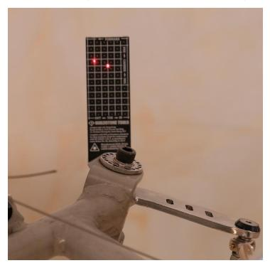
The setting shown shows *Toe* out and positive *Camber*. Now we can proceed to change the *Camber* and *Toe* out for either a new setting or to bring both sides of the cart to the same amount of *Toe* and *Camber*.
