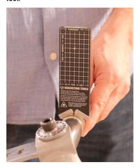
(3) Check level bubble and level the tool.
